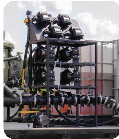
Direct inject herbicides into the carrier flow.
